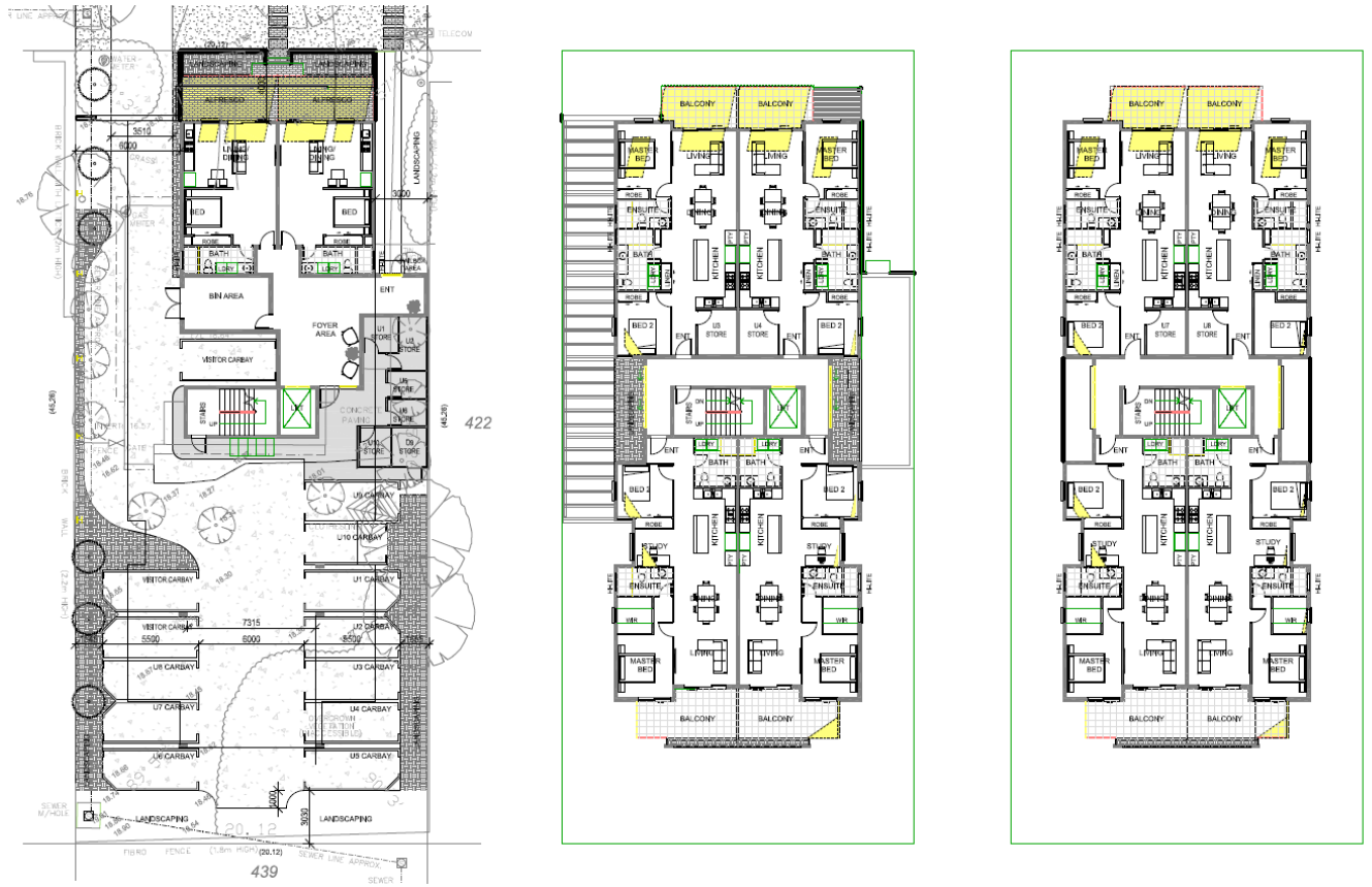
Figure 1: Solar access diagrams demonstrating 80% of the units receiving northern solar access. Only Unit 5 and 9 do not have direct sunlight to the living area.
