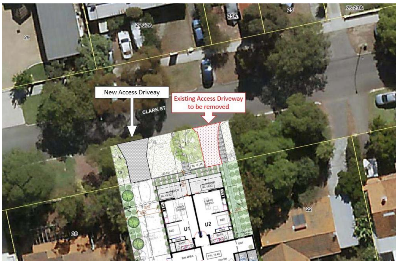
Figure 4 – Overlay of extract from development drawings with aerial photograph of site showing accesses
