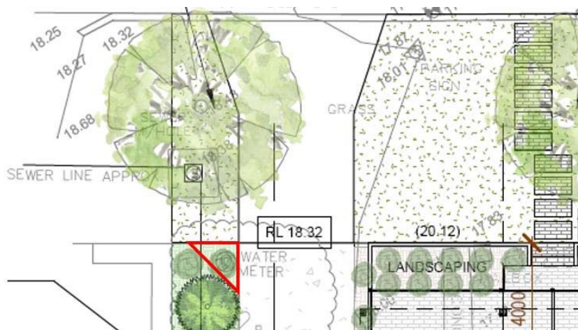
Figure 6 – Overlay of required truncation at driveway to provide sightline (bush to be removed)
