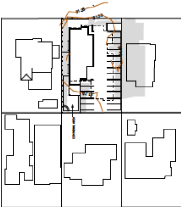
OVERSHADOWING AT 1:00PM JUNE 21st
