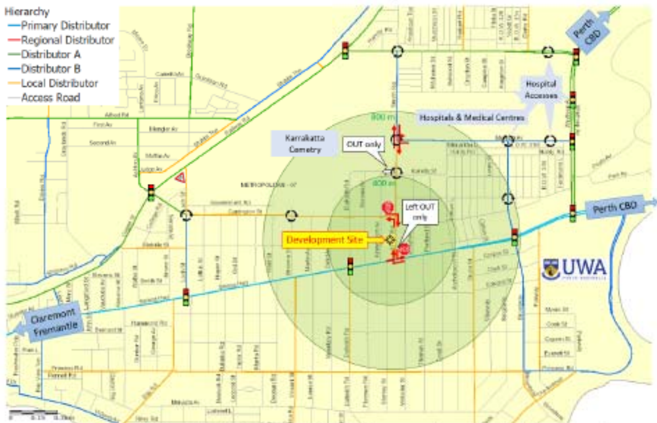
Figure 2 – Road Hierarchy, traffic control of access/ egress routes and context of surrounds
