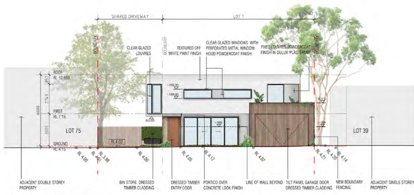
EASTERN ELEVATION (LOT 1 FENCE NOT SHOWN)
