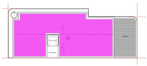
Note the image shows sufficient area for ~40kW peak output array.
