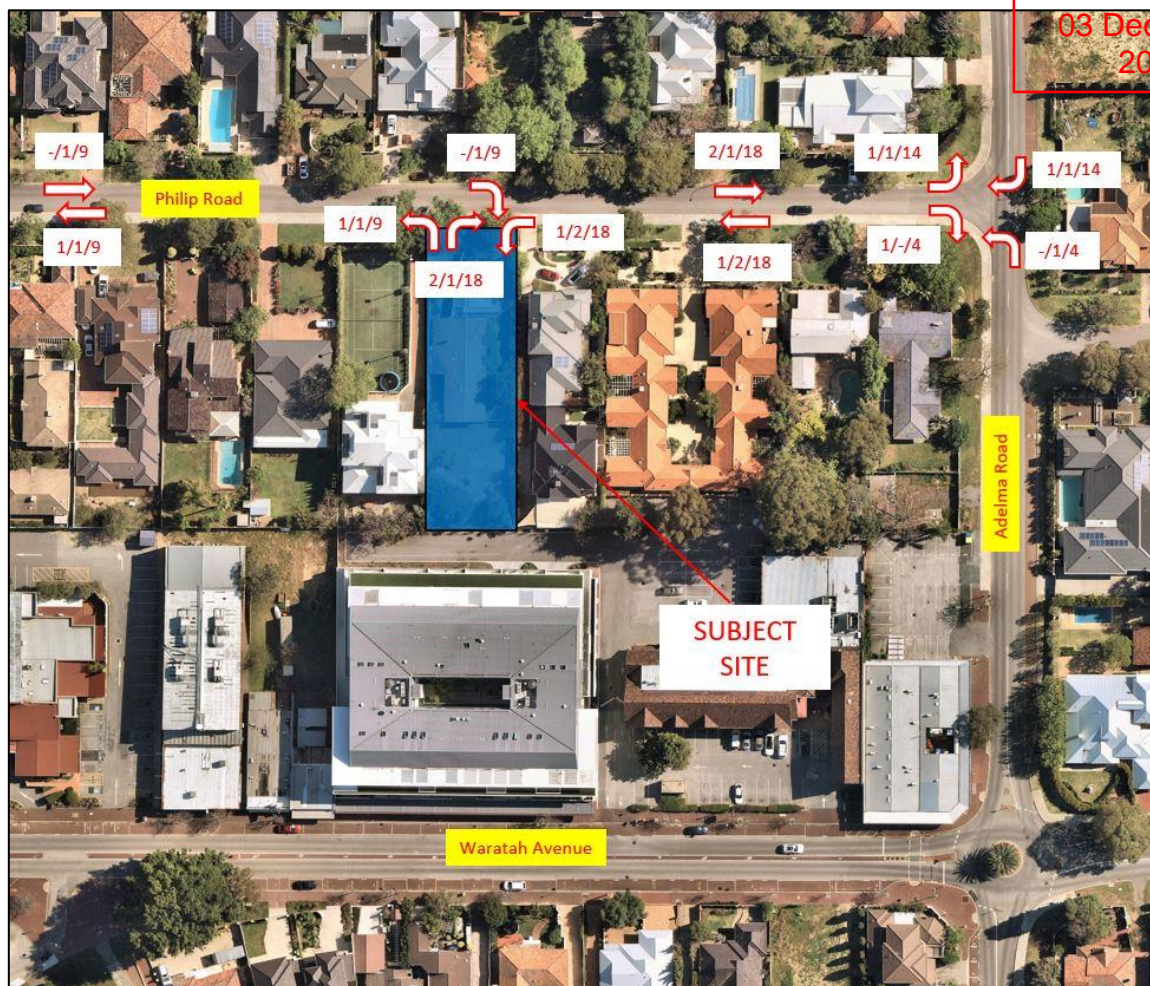
Figure 3. Estimated traffic movements for the subject development – morning, afternoon peak and total daily trips
