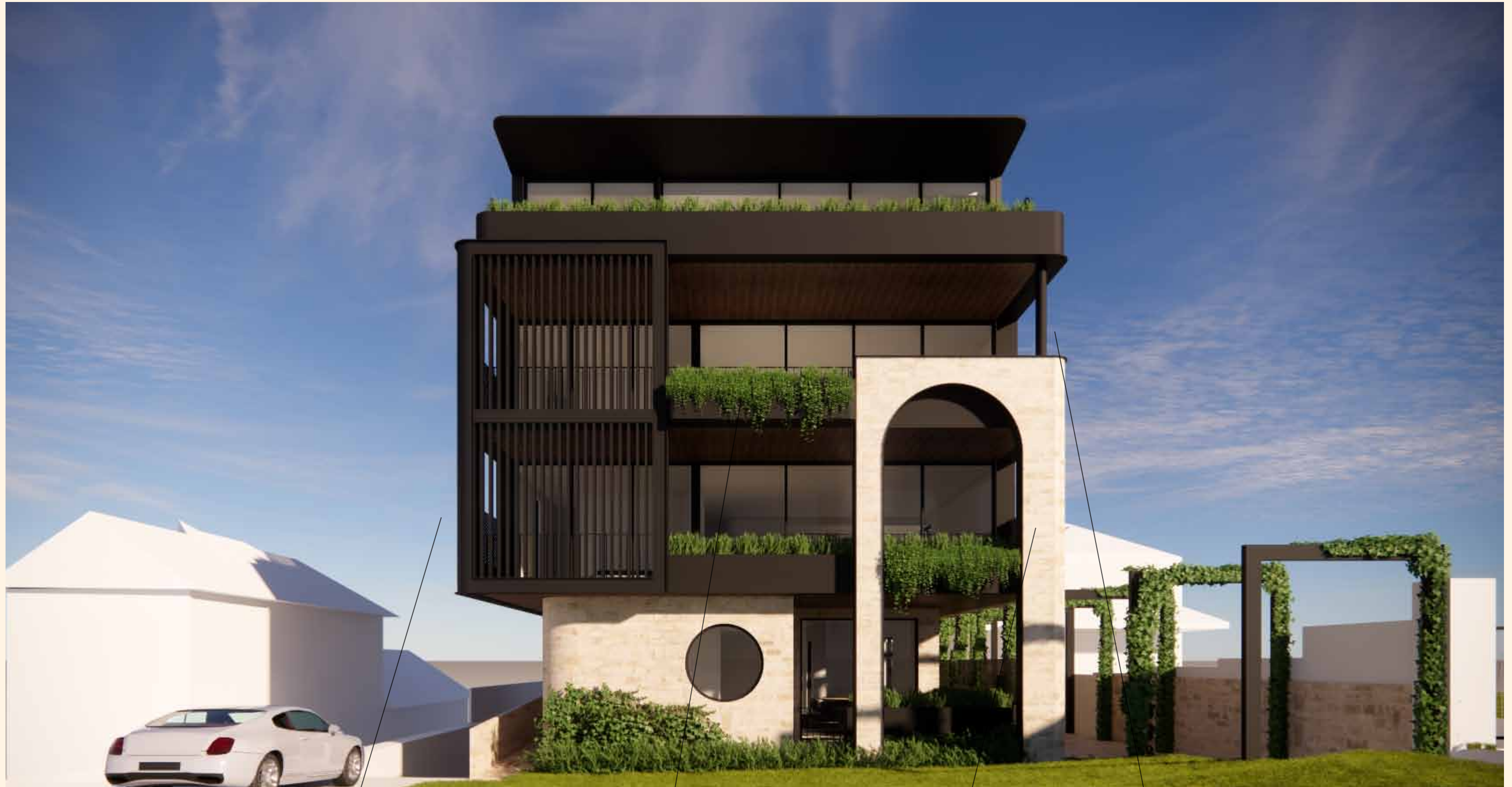
Corner column 'recessed' visually to prioritise perception and 'weight' of arched element
