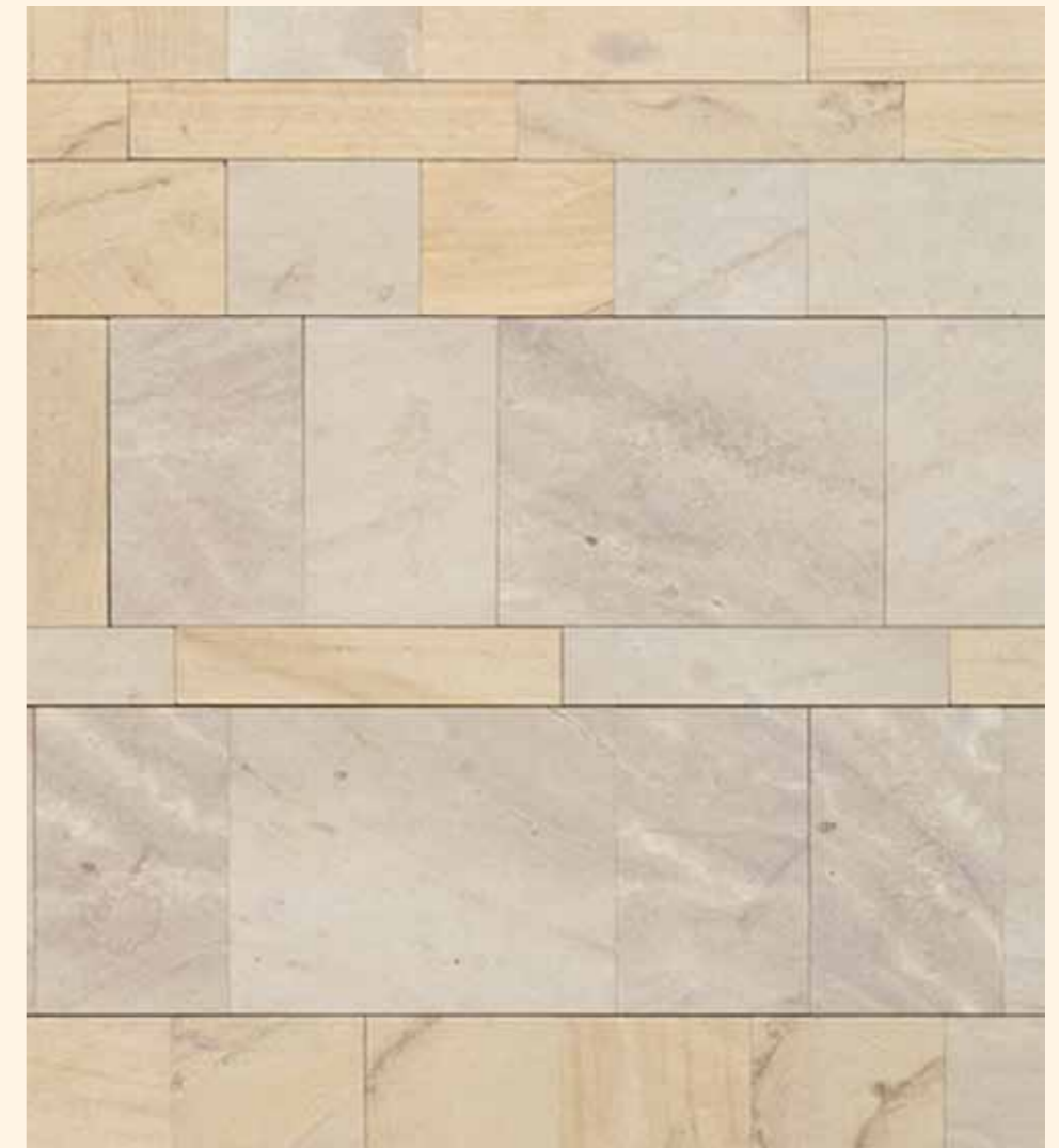
HONED LIMESTONE TILED CLADDING
