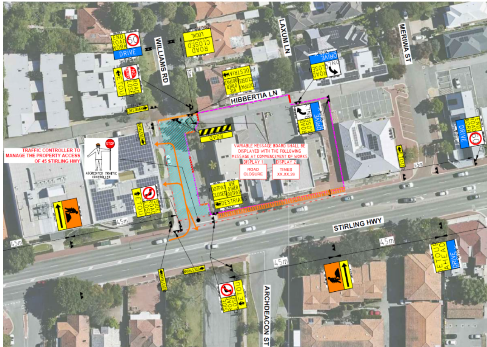
Figure 2 – Details of Proposed Closure Locations
