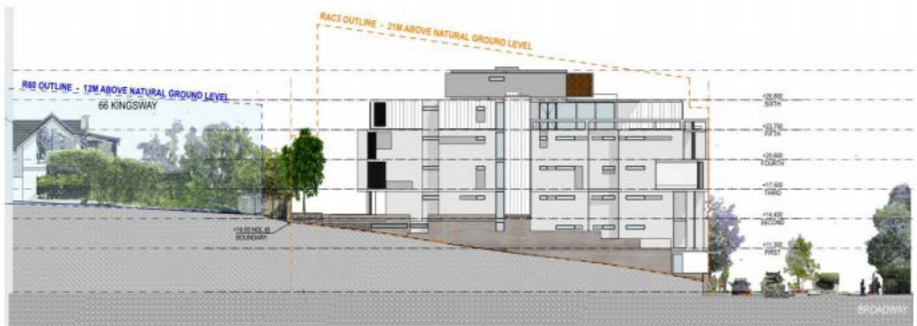
Section of development proposal at 135 Broadway depicting natural ground level and default height limit – source: MAARCH, March 2020
