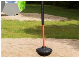
The specially designed seat is made from a stainless-steel insert covered with a soft layer of PUR rubber. The seat is impact tested to comply with global playground standards and the rope has an ergonomic handhold of a 60cm long moulded on PUR rubber handle.
