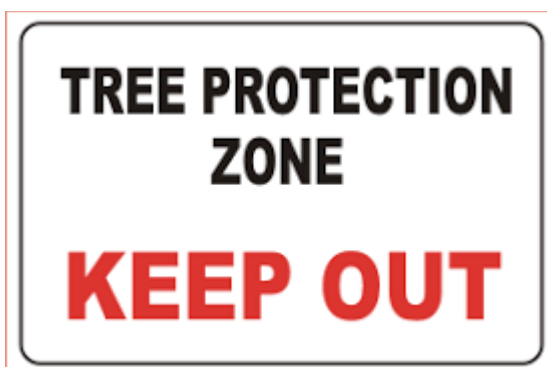
Fig. 5 – TPZ signage to be placed on fencing and visible to construction workers.
