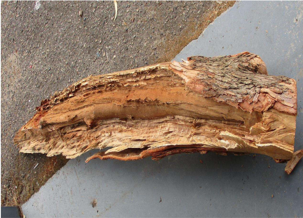
Figure 10 Displaying the failed stub section with no visible evidence of an internal defect contributing to failure.
