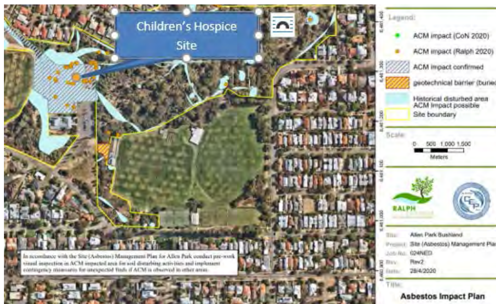
Figure 7: Allen Park Asbestos Impact Plan
