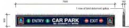
SIGN TYPE 3 (x1) CARPARK BULKHEAD SIGN (F17-BHCP) Single sided illuminated flexface wall sign.
