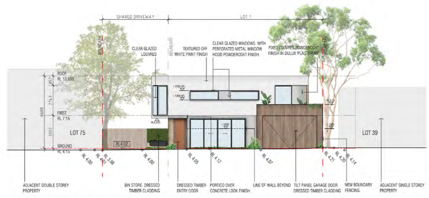
EASTERN ELEVATION (LOT 1 FENCE NOT SHOWN)
