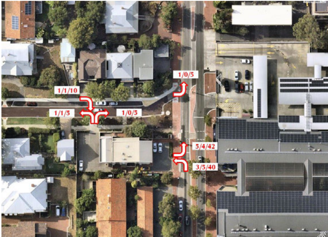
Figure 2. Estimated traffic movements for the subject development – morning, and afternoon peak hour trips
