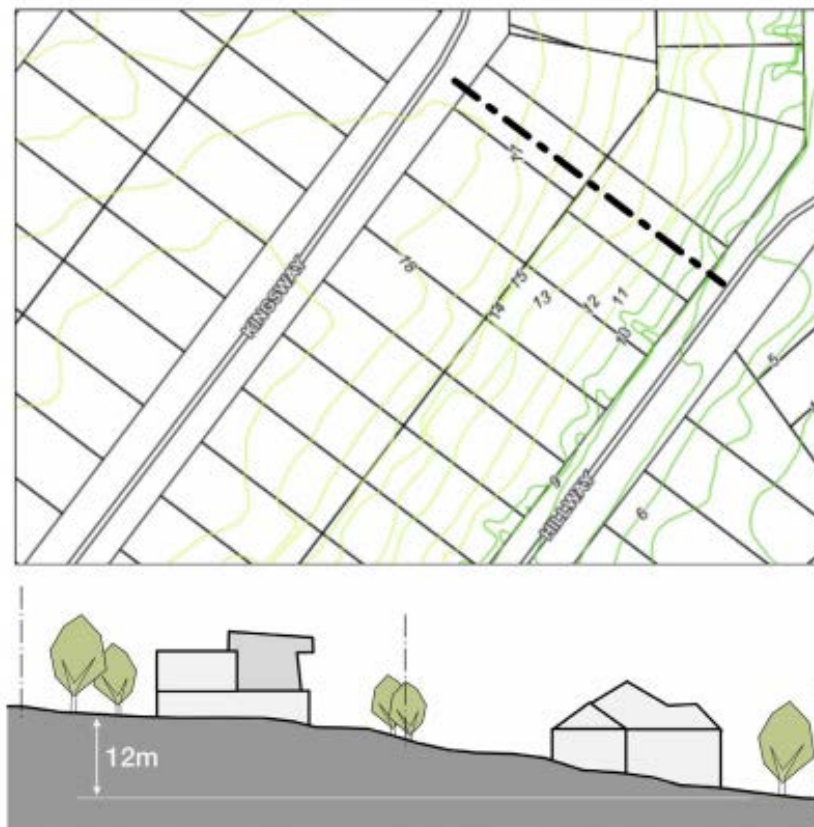
Contour map and cross section depicting typical change in elevation between Kingsway and Hillway – April 2020
