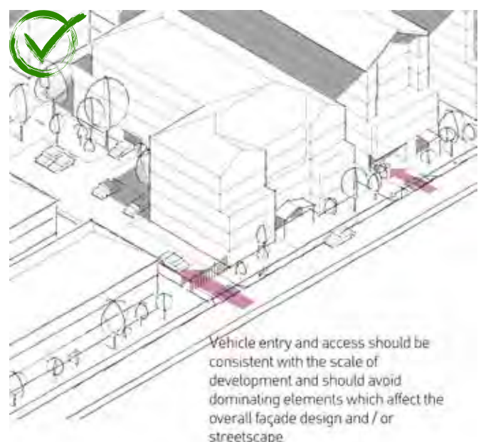
Figure 20. Multiple Dwellings - Vehicle Access Example Diagram
