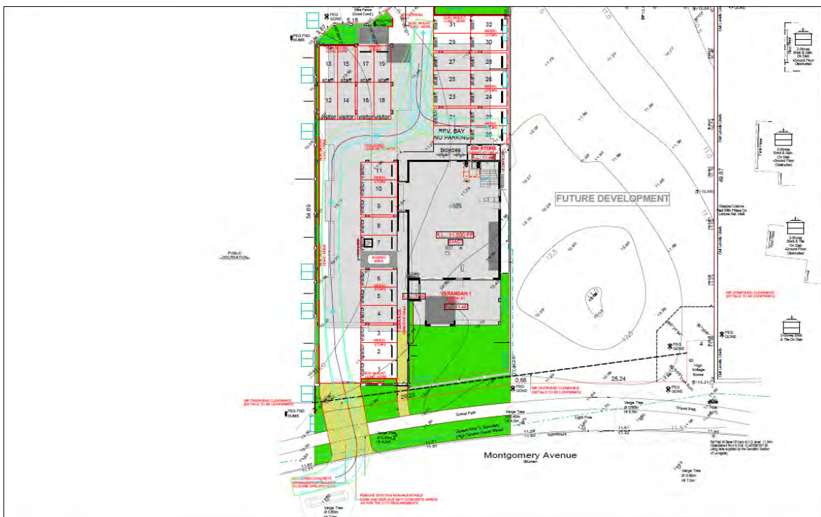
Diagram 1: Swept Path Analysis – Vehicle Entry
