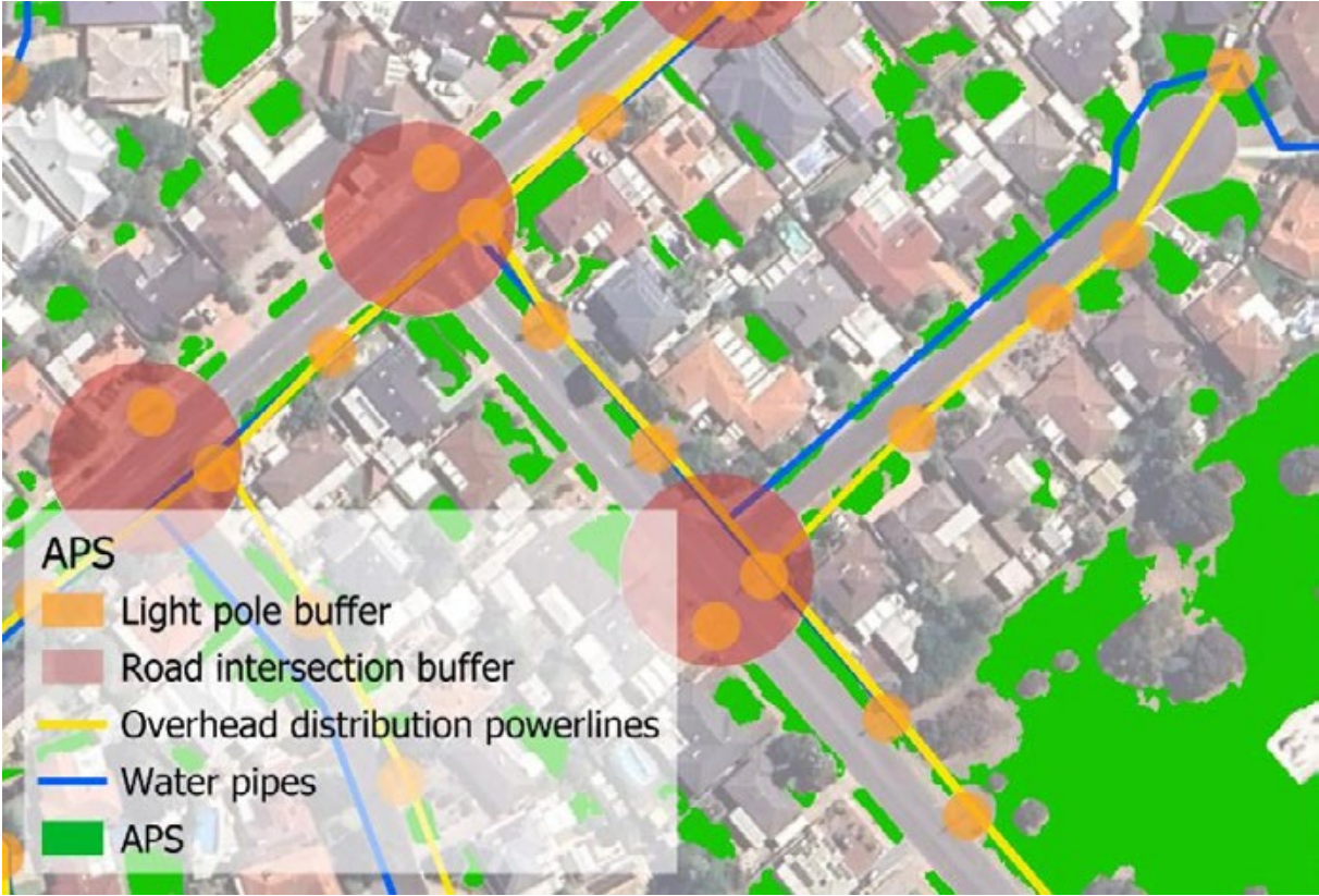
Figure 19. Available Planting Space (APS) and the limiting factors used to determine areas of APS.
