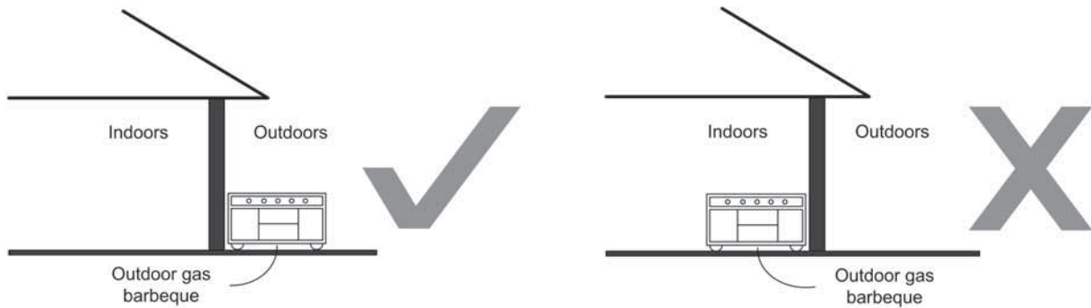
Figure 5a: Permanent structures - Examples of conforming (denoted with ✓) and non-conforming (denoted with X) installations
